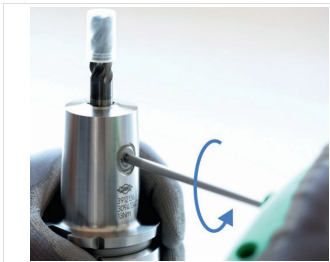
Fig. 6: Loosening clamping screw
