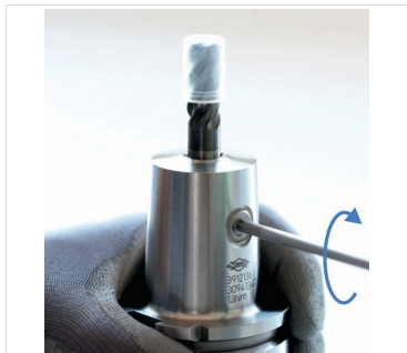
Fig. 5: Tighten the clamping screw to the prescribed tightening torque
