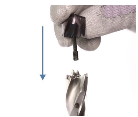
Fig. 6: Fit the replaceable drill head
