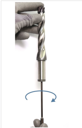
Fig. 12: Loosen replaceable drill head by turning in clockwise direction
