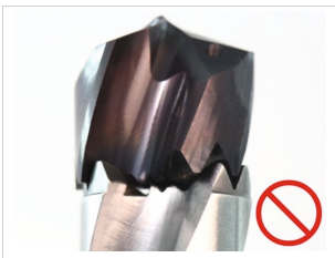
Fig. 7: Chip flute and serrations are aligned (left) | are not aligned (right)
