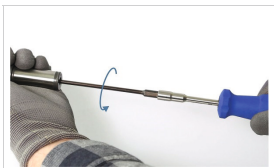
Fig. 11: Tighten the special clamping screw to the prescribed tightening torque
