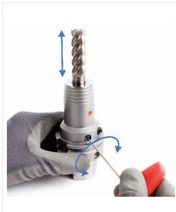
Fig. 11: Adjusting tool length (radial)
