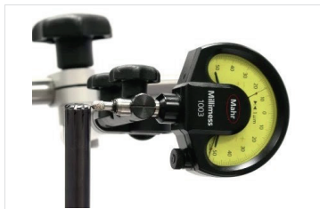
Fig. 16: Measuring the radial run-out
