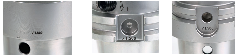
Fig. 5: Marking for checking of the clamping force: Three possible positions on the clamping chuck
