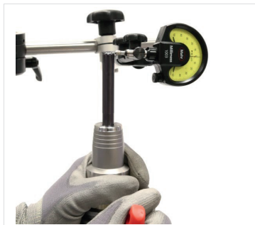
Fig. 17: Adjusting the radial run-out
