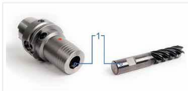
Fig. 7: Cleaning hydraulic chuck and tool
