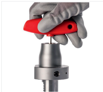
Fig. 8: Adjusting tool length (axial)
