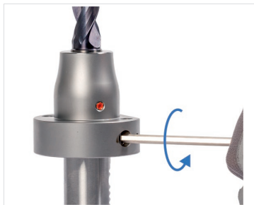
Fig. 12: Loosening clamping screw
