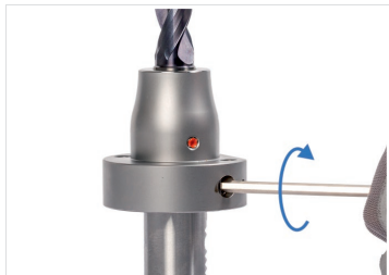
Fig. 11: Tightening clamping screw 2
