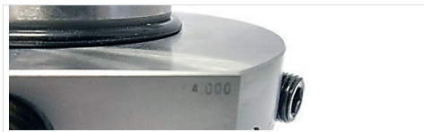
Fig. 5: Marking for checking of the clamping force
