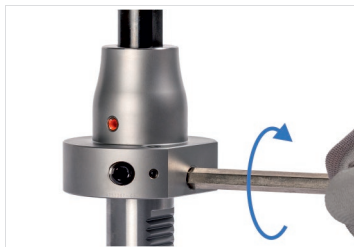
Fig. 15: Tightening locking screw
