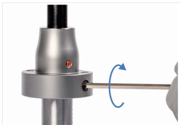
Fig. 16: Tightening clamping screw 2
