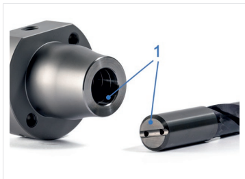
Fig. 7: Cleaning hydraulic chuck and tool
