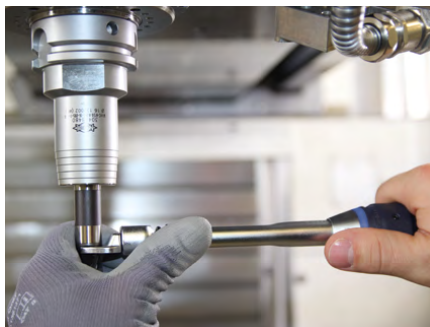
5. Note: Place your free hand on the replaceable milling head to be able to make delicate adjustments. This allows the tightening torque to be set more precisely.
