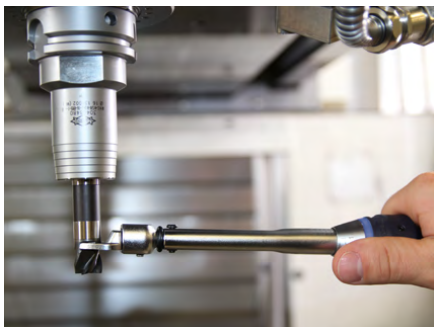
4. Place the torque wrench on the replaceable milling head so it is as horizontal as possible; do not tilt the faces on the wrench.
