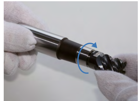
3. Hand tighten the replaceable milling head clockwise into the replaceable head holder. Then clamp the replaceable head holder with the tool in the machine holder.
