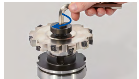
8. Screw in the milling cutter clamping screw further clockwise using a hex-wrench and then tighten it with a torque wrench (for tightening torque, see table "Tightening torque for milling cutter clamping screw").
